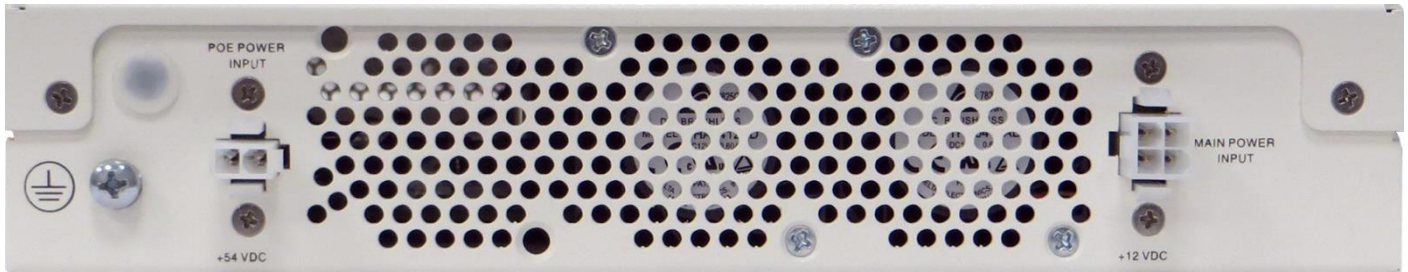
Figure 5. vE-CPE 1U Unit rear panel 54 VDC POE Power and 12 VDC Main Power
